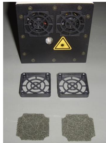
Figure 9: Replace filter mats
