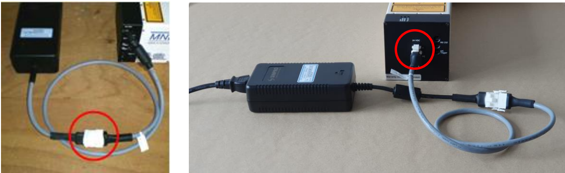
Figure 7: Connecting the mains
