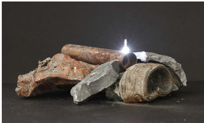
Classification of metals and alloys with LIBSorter AI based on laser-induced breakdown spectroscopy
