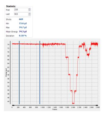
During a running measurement it may be useful to have the right cursor always being placed to the last measured value.
