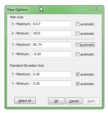
To manually change the scaling of the axis in your recording chart, click on either axis. The following dialog will show up.
