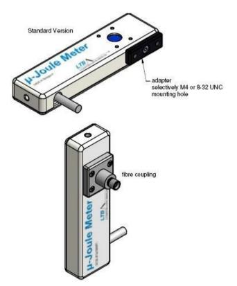
The adapter plate allows screwing a stand underneath the  $\mu$ -Joule Meter in order to achieve more stability during the measurement process; the plate contains two mounting holes, for metric or inch screws.
